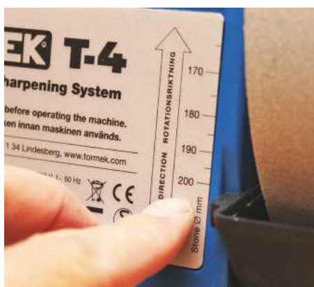
▲ You can check the wear of the stone against this simple diameter gauge
